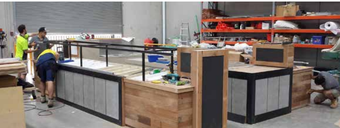
Construction phase of John's Nuts Kiosk, Kiosks are fully assembled in our facility prior to dispatch and onsite installation. This allows high quality assurance and minimises and eliminates any unknown compatibility issues on site, allowing a smooth transition from factory to site.
